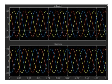
In this example, the **Component structure** parameter of the RLC block specifies that the electrical characteristics of the three-phase load are purely resistive. Therefore, for each phase of the three-phase system, the voltage and current remain in phase with each other. Because the resistance in each phase is  $\mathbf{1}\ \Omega$ , the magnitude of the phase voltage is equal to the magnitude of the phase current.
